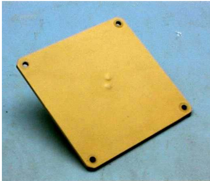
Figure 9. Single frequency Microstrip Patch Antenna.
