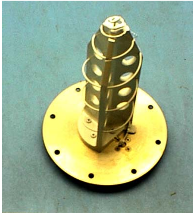
Figure 6. Genesis Spacecraft Medium Gain Antenna.
